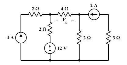
a. How many equations are necessary to analyze this circuit by the mesh analysis method?
